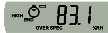
Highest reading of humidity sensor after logging has ended, upper alarm specification was exceeded, battery is low.
